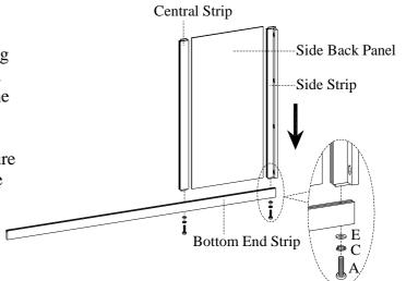
STEP 2: Then insert the central back panel with the cord hole in the bottom. Attach the top end strip to whole back panel using 4 bolts(A), lock washers(C) and flat washers(E). Make sure the back panels' finished side is facing inward. Completely tighten all bolts.
