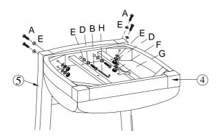
STEP 2: Attach Seating(4) to Chair back(5) by using bolts(A), bolts(B), lock washer(D), flat washer(E) and 4 hex nut(F), use Allen key(H) and hex wrench(G) tighten all bolts.
