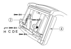
STEP 4: Place the Seating Unit(4) onto the Pneumatic Cylinder(1), aligning the top of the Pneumatic Cylinder(1) to the hole in the Seating Plate(2).
