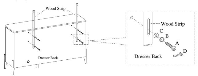
STEP 2: Attach the wood strip to the mirror by using 4 bolts(A), lock washers(B), and flat washers(C). Tighten all bolts on dresser and mirror with Allen wrench.
