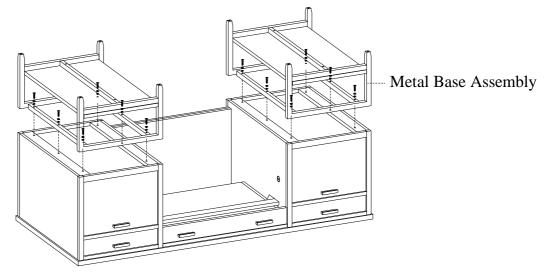
Notes: To reassemble desk, replace bolts removed in STEP 2 above before proceeding to STEP 3 below. Tighten all of the bolts completely.
