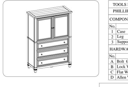
STEP 1: Put the case upside down on a soft surface, Attach the legs and support leg to the bottom of case by using 8 bolts(A), lock washers(B) and flat washers(C). Return the case to the upright position.
