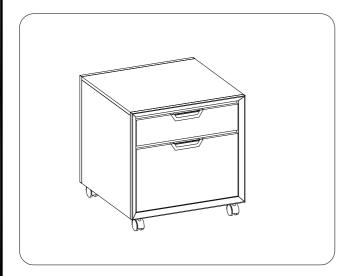
STEP 1: Put the case upside down on a soft surface. Attach the casters to bottom of the case use a hex wrench to tighten all the casters. Turn the case to the upright position.
