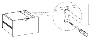
Remove the wood screws on the back panels of drawer box to remove the rod loops and file rods if necessary.
