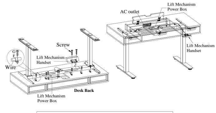
Note: Refer to Lift Mechanism assembly instructions for Handset operation.
