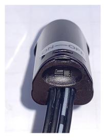
2. Slide switch on - Enable Ambient Light Detection When ambient light is detected, the PIR sensor does not activate.
