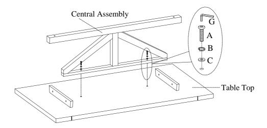
STEP 2: Attach the side assemblies to table top by using 4 bolts(A), lock washers(B), flat washers(C) and using 2 bolts(D), lock washers(E) flat washers(F) as shown below. Completely tighten all bolts. Turn the assembled table to the upright position.
