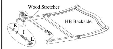
STEP 2: Attach the wood stretcher to the legs by using 4 bolts(I), lock washers(J) and flat washers(K).
