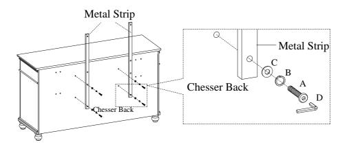
STEP 2: Attach the metal strips to the TV frame by using 4 bolts (A), lock washers (B) and flat washers (C). Tighten all the bolts on TV frame and Chesser with Allen wrench.
