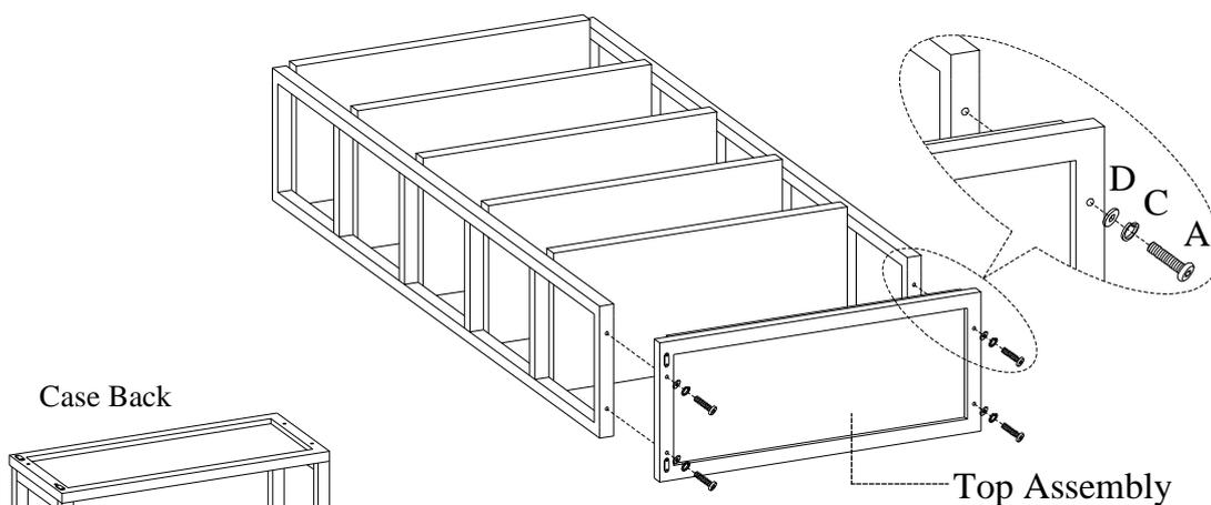
**STEP 4:** Place the metal stretchers on the back of the case assemble by using 4 bolts(B) and 1 wood screw(F), lock washers(C) and flat washers(D). Use the Allen wrench provided to tighten all the bolts.
