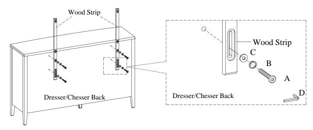
STEP 2: Attach the wood strips to the mirror back by using 4 bolts(A), lock washers(B), and flat washers(C). Tighten all bolts on dresser/chesser and mirror with Allen wrench.
