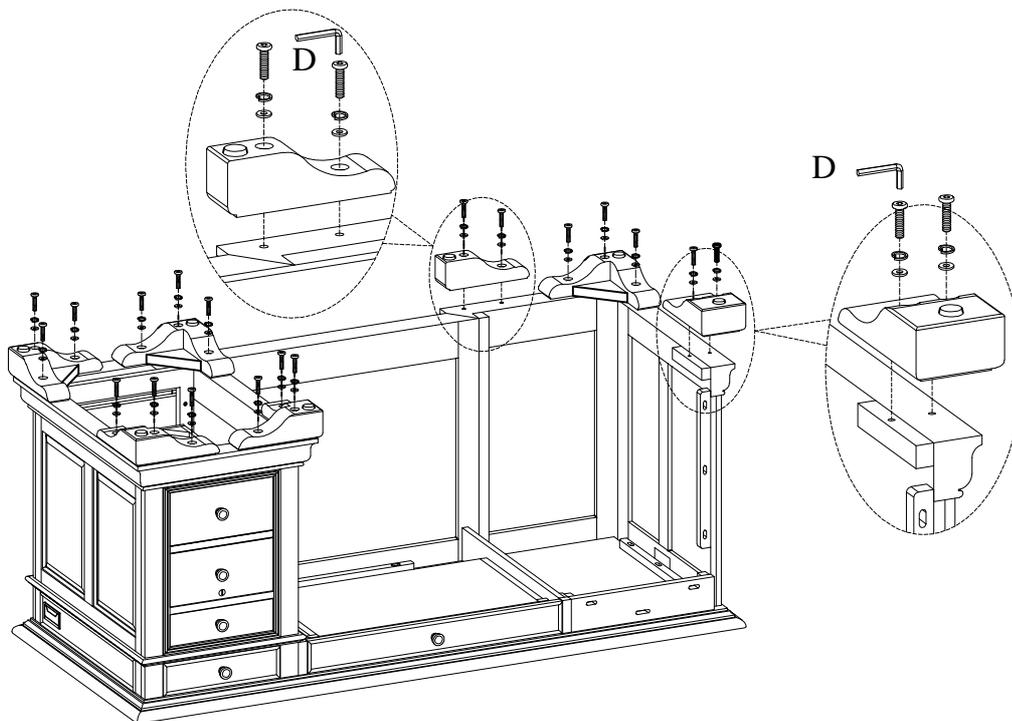
**STEP 1:** Align the holes in the desk end connector with the holes in the return. Use 6 bolts (A), lock washers (B) flat washers (C) to connect desk and return. Use an Allen wrench tighten all the bolts.
