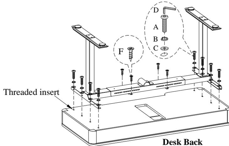
**STEP 4:** Tighten bolts that were loosened in Step 3 from the IUAB-301-1 assembly instructions.
