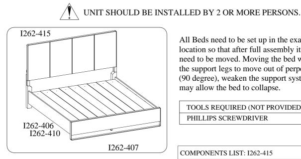
HARDWARE LIST: I262-415 Description No. Quantity Sketch A | Bolt Ø5/16" x 1-3/4" 8 PCS В Lock Washer Ø5/16" Ð 8 PCS С Flat Washer Ø5/16" x 3/4" 0 8 PCS D Allen Wrench 5mm 1 PC
