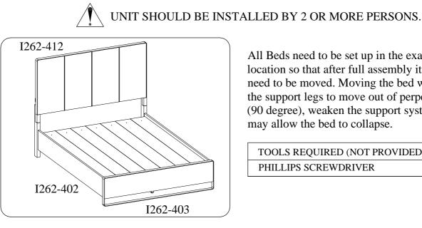
All Beds need to be set up in the exact final location so that after full assembly it will not need to be moved. Moving the bed will cause the support legs to move out of perpendicular (90 degree), weaken the support system, and may allow the bed to collapse.
