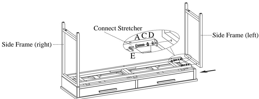
**STEP 4:** Attach the support stretchers to table assembly by using 4 bolts(A), lock washers(C) and flat washers(D). Then use an allen wrench to tighten all the bolts.
