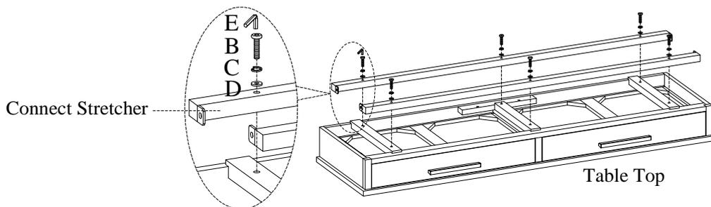
**STEP 3:** Attach side frames (left & right) with "L" and "R" markings to connect stretchers by using 4 bolts(A), lock washers(C) and flat washers(D). Do not completely tighten bolts.
