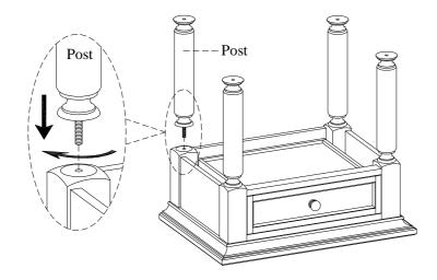
STEP 3: Attach the bottom shelf to the posts with bun feet as shown below. Turn the assembled case to the upright position.
