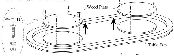
STEP 3: Attach the wood plates to the pedestals by using 8 bolts(A), lock washers(B) and flat washers(C) with the allen wrench(D). Completely tighten all the bolts.
