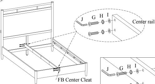
STEP 3: Attach 3 support legs (for center rail) to the center rail using 6 bolts (G), lock washers (H) and flat washers (I). Use the allen wrench (J) to tighten all of the bolts.
