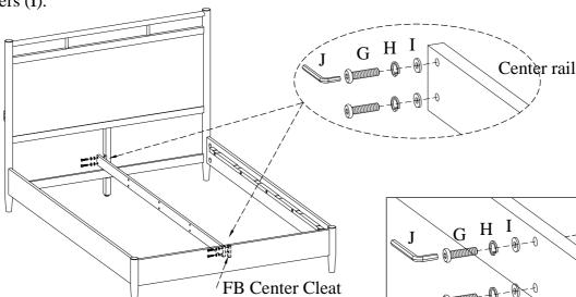
STEP 3: Attach 3 support legs (for center rail) to the center rail using 6 bolts (G), lock washers (H) and flat washers (I). Use the allen wrench (J) to tighten all of the bolts.
