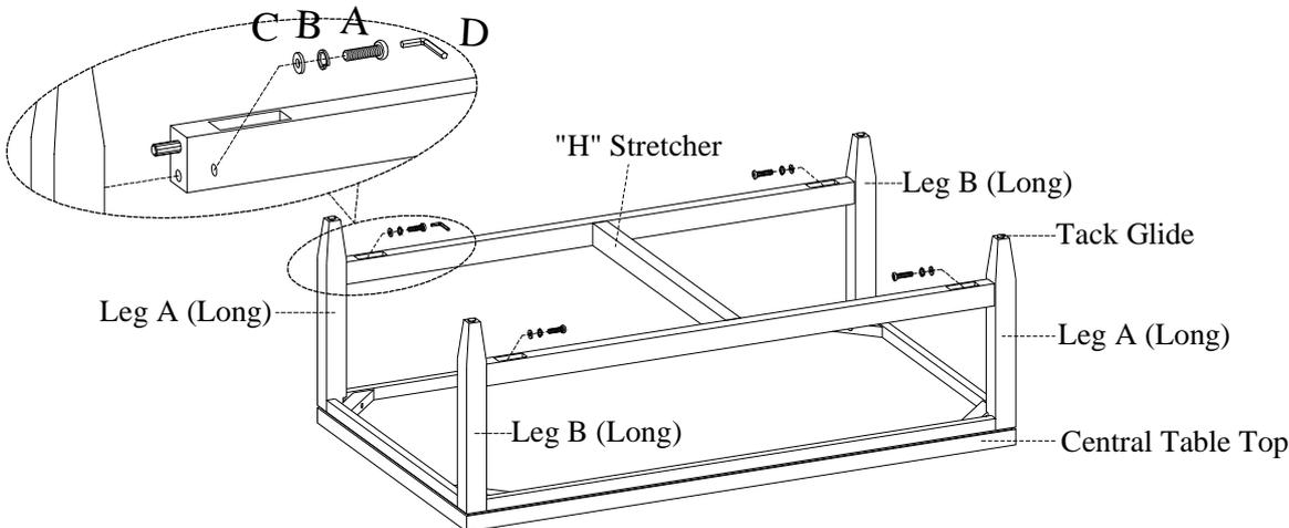
**STEP 2-2:** Attach the bottom shelf to the legs by using 4 bolts (A), lock washers(B) and flat washers(C). Completely tighten all bolts. Turn the assembled table to the upright position.
