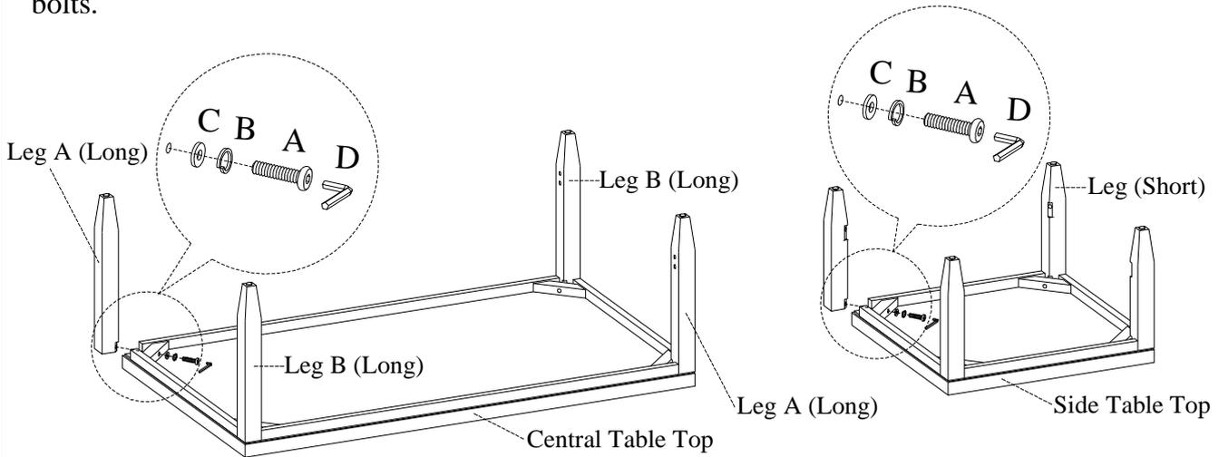
**STEP 2-1:** Attach the "H" stretcher to the legs by using 4 bolts (A), lock washers(B) and flat washers(C). Completely tighten all bolts. Turn the assembled table to the upright position.
