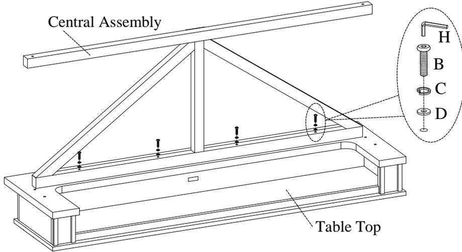
**STEP 2:** Attach the left/right side assemblies to table top by using 4 bolts(A), lock washers(C), flat washers(D) and using 2 bolts(E), lock washers(F) flat washers(G) as shown below. Completely tighten all bolts. Turn the assembled table to the upright position.
