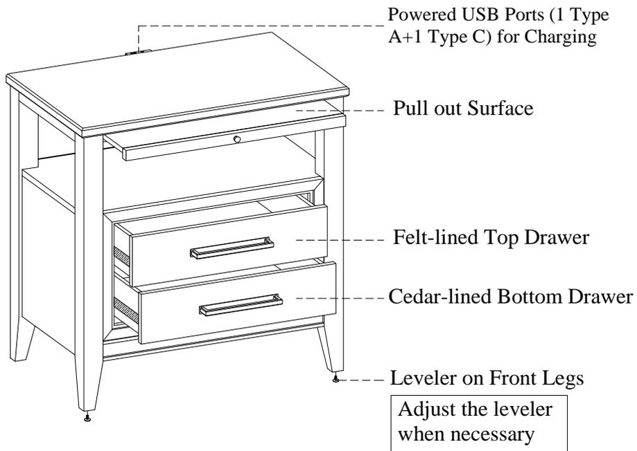
Adjust the leveler when necessary
