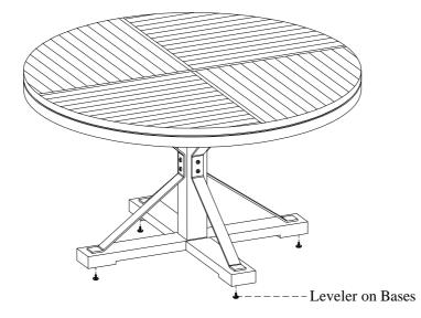
Adjust the leveler when necessary
