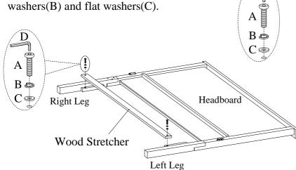
STEP 2: Attach the wood stretcher to the legs by using 2 bolts(A), lock washers(B) and flat washers(C).
