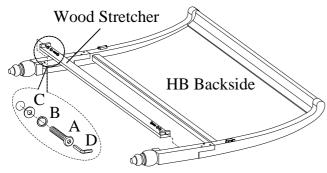
STEP 2: Attach the wood stretcher to the legs by using 2 bolts(A), lock washers(B) and flat washers(C).
