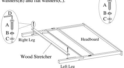
STEP 2: Attach the wood stretcher to the legs by using 2 bolts(A), lock washers(B) and flat washers(C).
