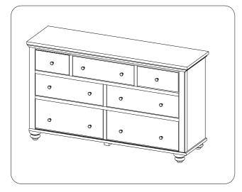
STEP 1: Put the case top face down on a soft surface, Attach the bun feet and support leg to the bottom of case, return the case to the upright position.
