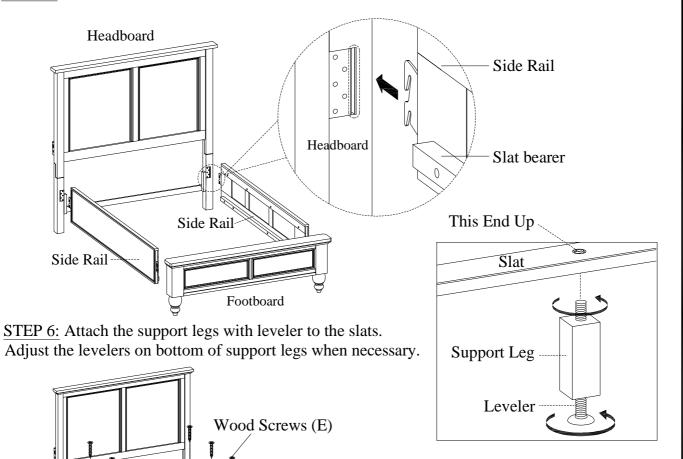
STEP 7: Arrange the slats on the slat bearers equally and attach to the slat bearers with wood screws (E).
