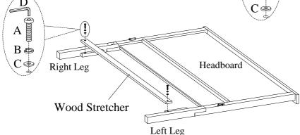
STEP 2: Attach the wood stretcher to the legs by using 2 bolts(A), lock washers(B) and flat washers(C).
