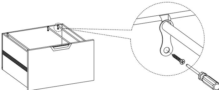
Remove the wood screws on the back panels of drawer box to remove the rod loops and file rods if necessary.
