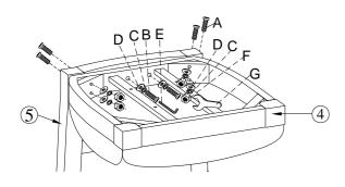
STEP 2: Attach Seating (4) to Chair back (5) by using bolts (A), bolts (B), lock washer (C), flat washer (D) and hex nut (F), use Allen key (E) and hex wrench (G) tighten all bolts.
