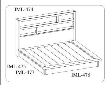
All Beds need to be set up in the exact final location so that after full assembly it will not need to be moved. Moving the bed will cause the support legs to move out of perpendicular (90 degree), weaken the support system, and may allow the bed to collapse.
