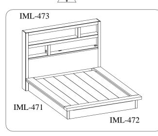
All Beds need to be set up in the exact final location so that after full assembly it will not need to be moved. Moving the bed will cause the support legs to move out of perpendicular (90 degree), weaken the support system, and may allow the bed to collapse.
